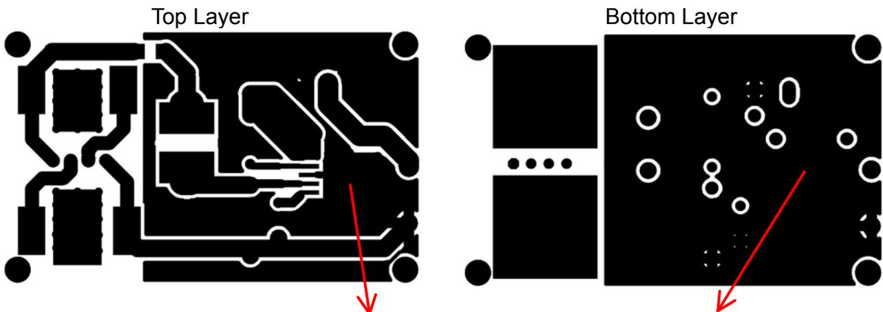
Large PCB area is reserved for GND plane and is connected to the heat pad of AMC7150. The GND plane can be a part of heat sink for AMC7150.
