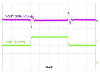
Figure 17. Load Transient, IOUT = 50mA to 500mA to 50mA
