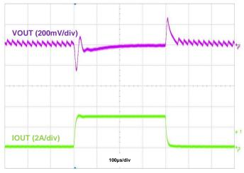
Figure 19. Load Transient, IOUT = 50mA to 3A to 50mA
