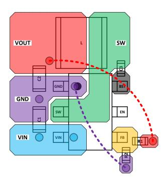
Figure 27. Recommended PCB Layout for SOT563 Package
