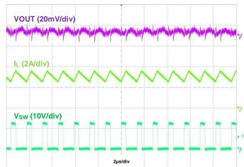
Figure 15. Output Voltage Ripple, VOUT = 3.3V, IOUT = 50mA
