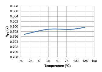
Figure 7. Feedback Voltage vs. Temperature
