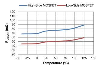
Figure 8. Power MOSFET  $R_{DS(ON)}$  vs. Temperature
