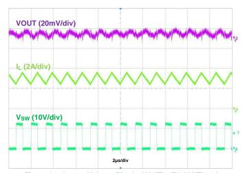
Figure 14. Output Voltage Ripple, VOUT = 5V, IOUT = 3A
