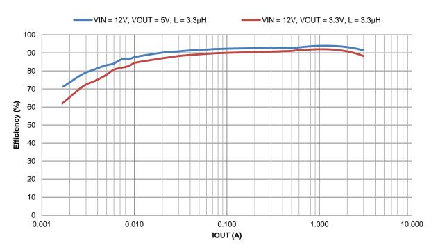
Figure 2. AP62300 Efficiency vs. Output Current
