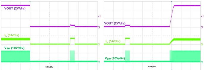
Figure 22. Output Short Protection, IOUT = 3A
