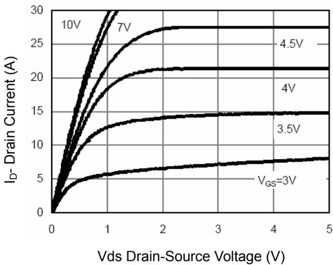
Figure 3 Output Characteristics
