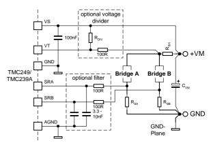
shunt resistor. Place the optional shunt resistor voltage divider near the TMC249, in order to avoid voltage drop in the VCC plane to add up to the measured voltage.
