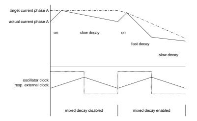
When polarity is changed on one bridge, the PWM cycle on that bridge becomes restarted at once.
