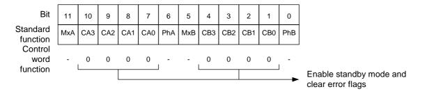
Programming current value "0000" for both coils at a time clears the overcurrent flags and switches the TMC249 into a low current standby mode with coils switched off.
