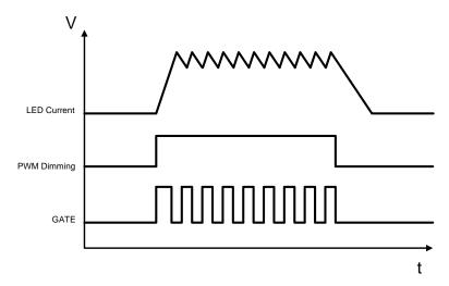
The rising and falling edges are limited by the current slew rate in the inductor. The first switching cycle is terminated upon reaching the 250 mV ( $V_{\text{DIM}} \cdot 0.167$ ) level at CS. The circuit is further reaching its steady-state within 1 switching cycles regardless of the switching frequency.
