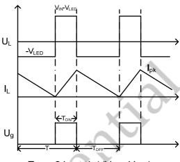
$T_{ON} = 2 I_{LED} \times L / (V_{IN} - V_{LED})$
